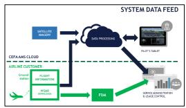
Fig. 1: QAR data processing for both mobile service and FDM program. (Courtesy CEFA Aviation)
